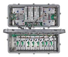
As the focus of a fiber deep collector node topology, the SG4000 supports advanced modules such as optical amplifiers, optical switches and ruggedized optical passives. The node accepts the new DOCSIS based status monitor transponder to allow operators to monitor and control node parameters using their existing DOCSIS infrastructure.
